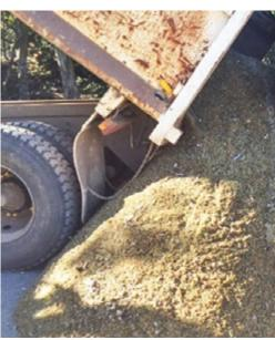
The other great thing about recycling glass this way is we can capture more products. Conventional glass recycling has only ever allowed for the recycling of glass jars and bottles, whereas when we crush it into sand, we can repurpose glass bottles and jars as well as plate glass, drinking ware, crockery and pyrex.
