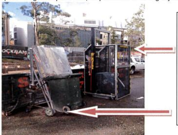
As you can see the unit is of a solid well built structure with full screening containment to catch any falling objects
